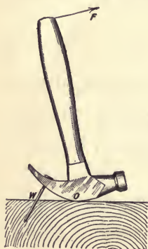
FIG. 53.—The Hammer used as a Bent Lever.
